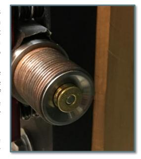
Lubricated cases can also produce erratic muzzle velocity even when the pressure is low enough to avoid case head swelling. The reason for this is not known with certainty but a possible explanation is that when the pin strikes the primer, the case moves forward (depending on available headspace) leading to a weak primer strike and lower muzzle velocity (about 20 fps for 308).
